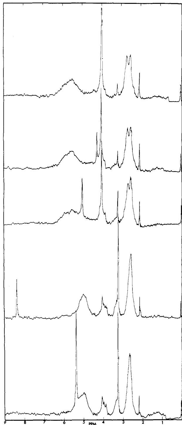
Figure 1. Pmr spectra of the hydrolysis products from [\text{Co}(\text{en})_2(\text{glyOCH}_3)](\text{ClO}_4)_3 in dimethyl sulfoxide- d_6 containing a trace of residual water after 5 min, 35 min, 85 min, 8 hr, and 8 hr (water added), respectively (internal reference, tetramethylsilane).
